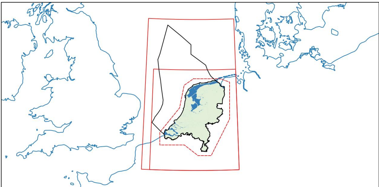
Figure 1.1.1. Validity area of RDNAPTRANS™ versions 2000, 2004 and 2008 (dashed red line) and bounds of the RDNAPTRANS™2018 grids and dense subgrid of the NTV2 file format (solid red lines) relative to the administrative borders and EEZ of the Netherlands (coloured area and black lines).
